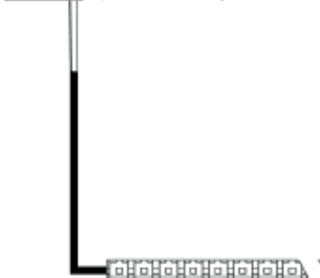
10 ft. wire harness with 12 pin connector
